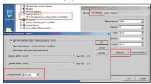
4.Open the BLHELISUITE, Select SILABS BLHeli Bootloader (Cleanflight) from the third tab on the top side. Then Select the right Serial com port and Click connect. You can also Flash the new release BLHeli\_s firmware via the BLHEILISUITE, the firmware Target is "O-L-05"
