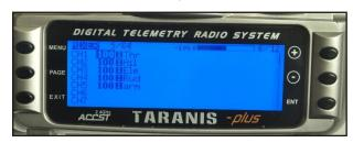
3. The default channel map for Snapper 6 Frsky version is TAER1234, please make sure your transmitter is matched, otherwise it will can't be armed. Toggle the AUX1 Switch, the Green LED on the flight controller will getting to be solid, this indicates the motor was armed. And also you can found "Armed" displayed on your FPV Goggles or the FPV Monitor. Please make sure keep the Snapper 6 level before arming. Be careful and enjoy your flight now!
